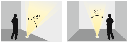
Asymmetrische Linse 45°/35° / Asymmetrical lens 45°/35°
