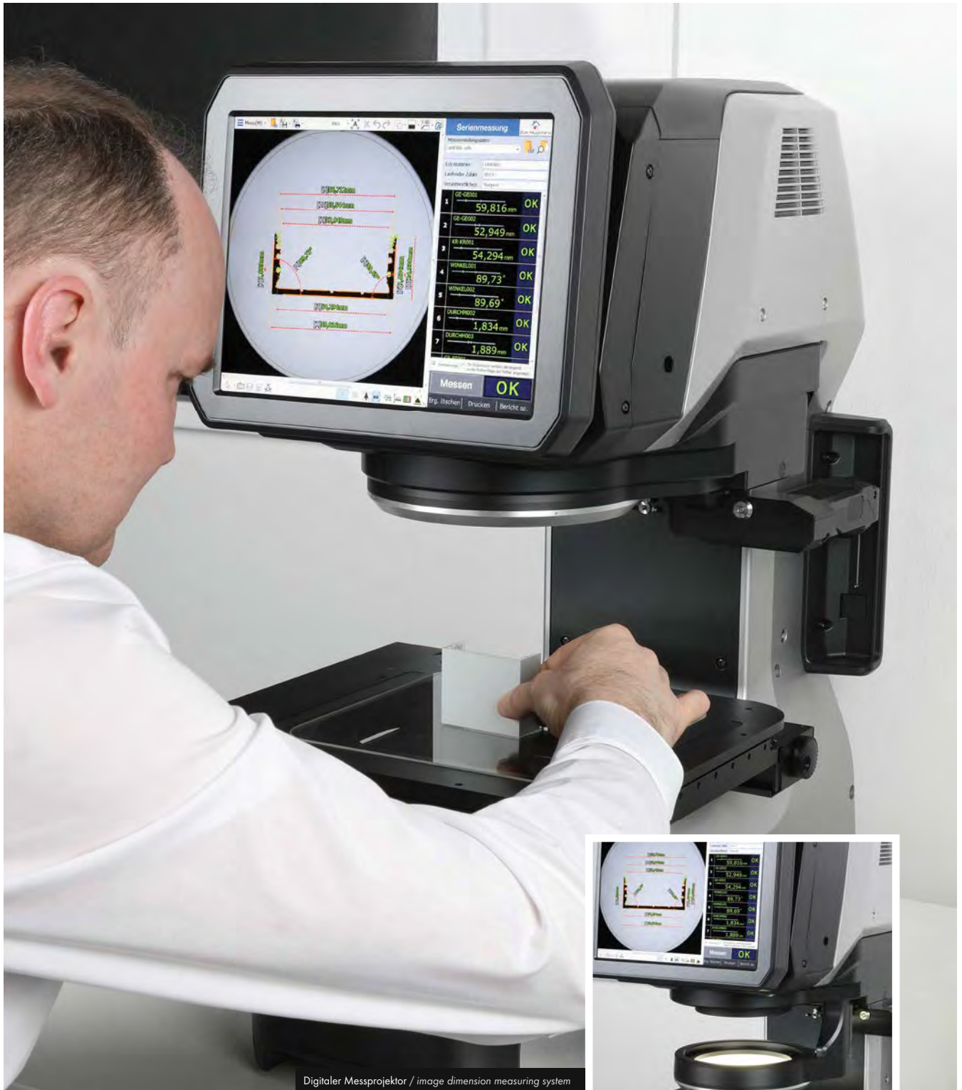
Digitaler Messprojektor / image dimension measuring system
